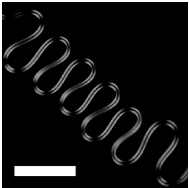
FIG. 1. Periodic buckling of a smectic-A filament observed at 41.0^\circ\text{C} with polarizer and analyzer crossed. The cooling rate was -0.05^\circ\text{C}/\text{min} . The bar indicates 50\text{ }\mu\text{m} .
